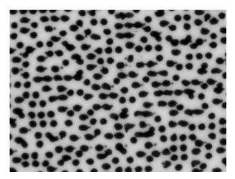
Figure 2a. High magnification image of a halftone printed on a glossy substrate
