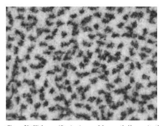
Figure 2b. High magnification image of the same halftone printed on a plain, uncoated substrate
